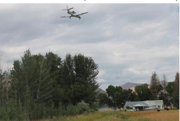
PHOTO 1 - OBSTRUCTIONS TO BE REMOVED- (TREE BELOW AIRCRAFT HAS A LIGHTING BEACON)
