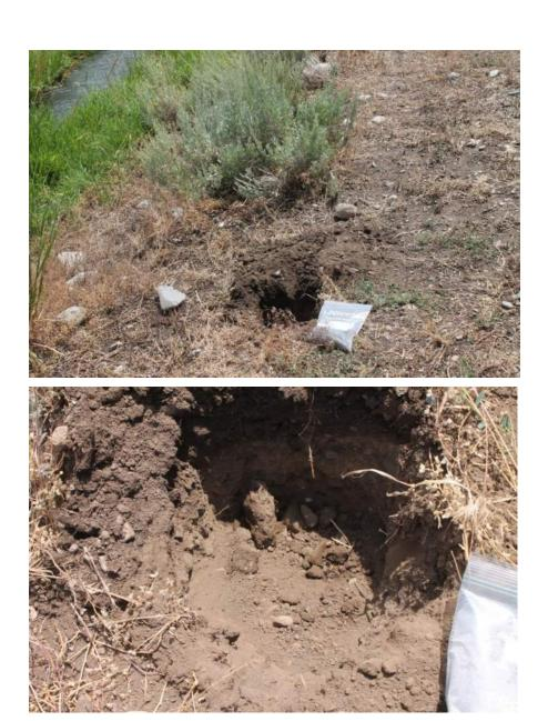
**PHOTO POINT 4:** Photo facing southeast at **SAMPLE POINT 3**, upland. Photo shows western end of wetland WL-1 which is approximately 5 feet from the Cove Canal at top of bank, spreading upland into Yellow Rabbitbrush (Chrysothamnus viscidiflorus) and upland pasture grasses. Soils 6-8" deep were dry sandy cobble with no redox
