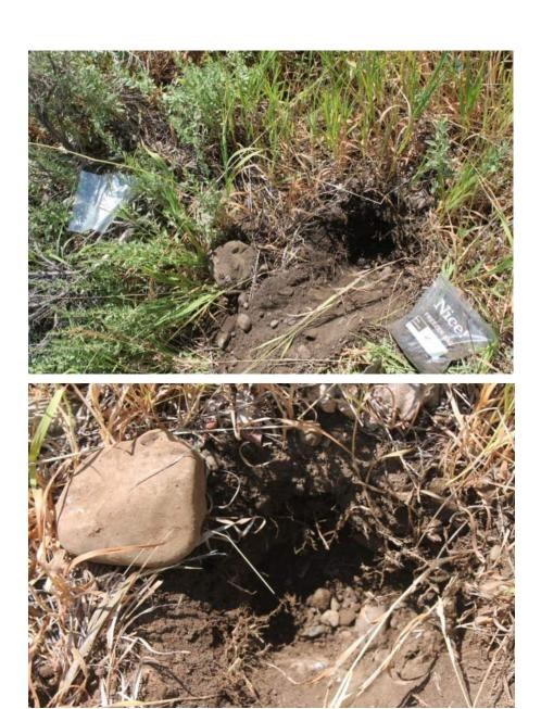
**PHOTO POINT 13:** Photo facing south on the west bank of the Cove Canal at **SAMPLE POINT 1** (WL-2). Soil had immediate refusal due to rocks, base was sandy-loam with cobble, sagebrush, thistle, wildrye, and reedgrass in the upland area.
